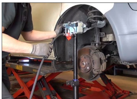
2. Pre-tension springs directly on the vehicle
