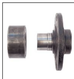
Two-piece standard wheel bearing
