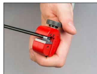
Positioning of line to scrape the covering
